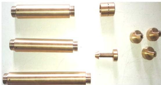
Fig.3 Photographs of double inlet nozzle vortex tube
