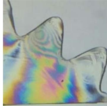
Figure 8 - Fringe pattern for Cosine gear
