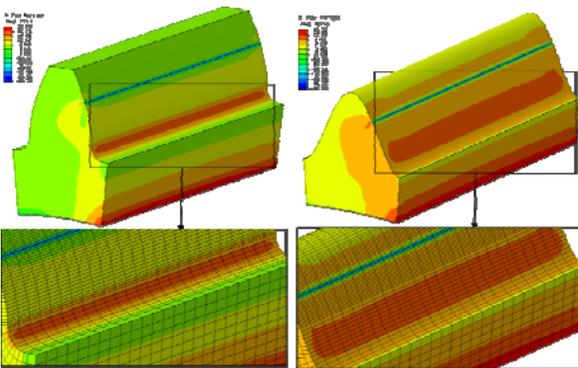
Figure 11 - Max. Principal Stress - Involute Gear and Cosine Gear
