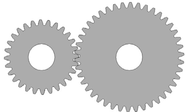
Figure 1 - CAD Model of Involute Profile Spur Gear
