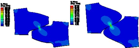
Figure 10 - von Mises stress - Involute Gear and Cosine Gear
