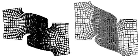
Figure 4 - Meshed models of Involute and Cosine gears
