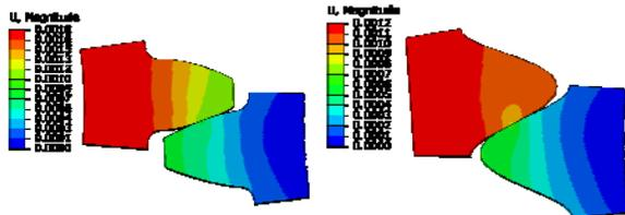
Figure 9 - Resultant deformation - Involute and Cosine Gear
