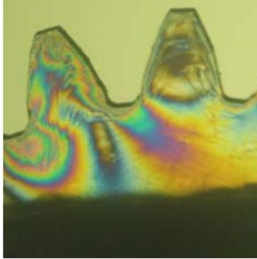
Figure 7 - Fringe pattern for Involute gear
