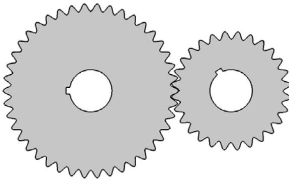
Figure 2 - CAD Model of Cosine Profile Spur Gear
