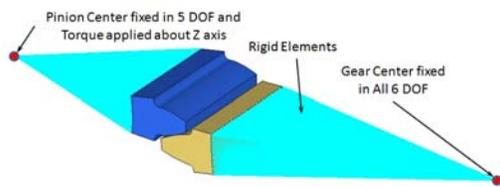
Figure 5 - Loading and Boundary conditions
