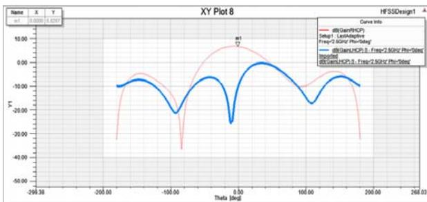
Fig.6. Gain LHCP and RHCP at 2.45GHz with Phi=0°
