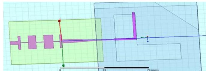
Fig.3. The Antenna with Filter
