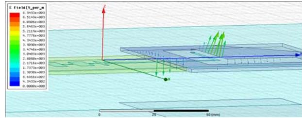
Fig.8. Vector E Field Patterns of antenna with filter
