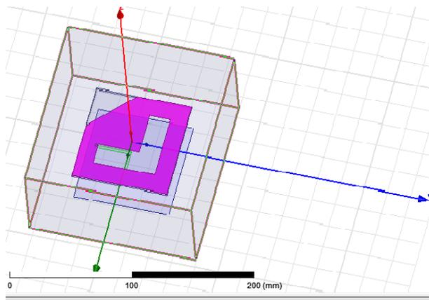
Fig.1. The Square Patch CP antenna structure.
