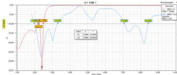
Fig.5. Combined frequency of antenna & filter in term of Return Loss
