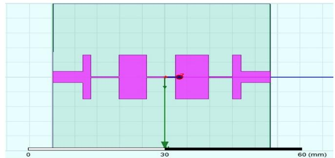
Fig.2. The Butterworth Low Pass Filter
