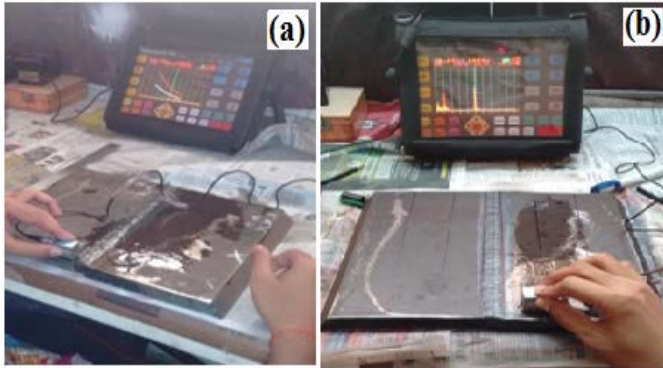
Fig.3. Ultrasonic testing of the weldments (a) SMAW (b) TIG
