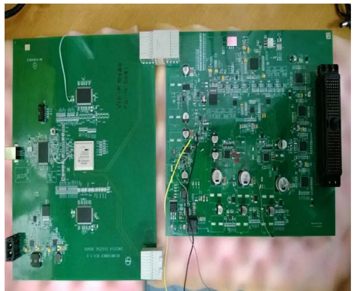
Fig 17:Hardware Build for the beamformer
