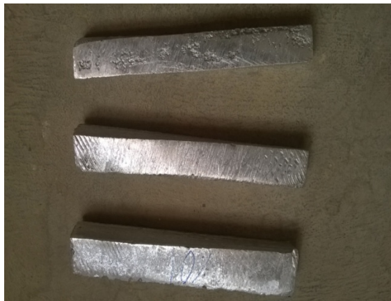
Fig 8 Impact & torsion test specimens
