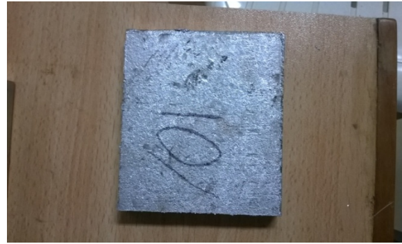
Fig7(b) Al - 10% of sic p hardness test specimen
