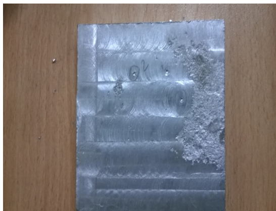
Fig 7(a) Al - 5% of sic p hardness test specimen
