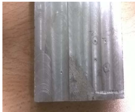
Fig 7 (c) Al - 15% of sic p hardness test specimen
