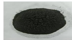
Fig.2. Silicon carbide (SiC) with a particle size of 30 μm
