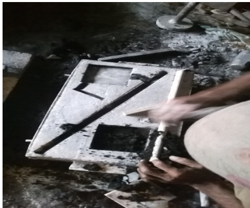
Fig3(a).Pattern making for test specimen
