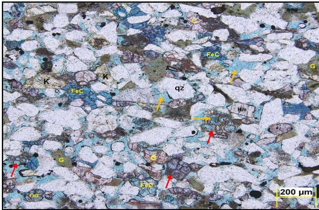
Fig. 9 Mineralogical Composition Thin Section of Nukhul-C (Core Sample).
