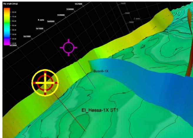
Fig.6: Calculated fault dip for the Buselli faults
