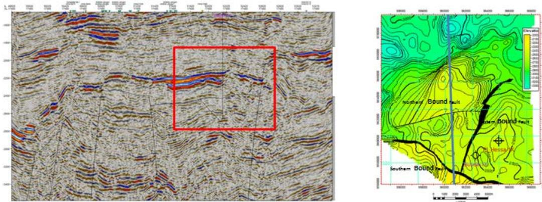
Fig.3: seismic line & Structure map of top 6.8 SB with main bounding faults
