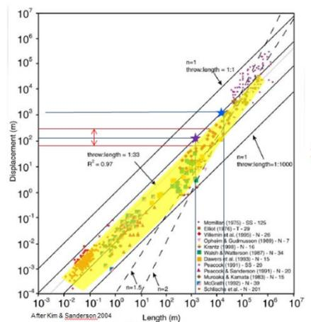
Fig.5: Fault length/displacement relationship for Buselli fields
