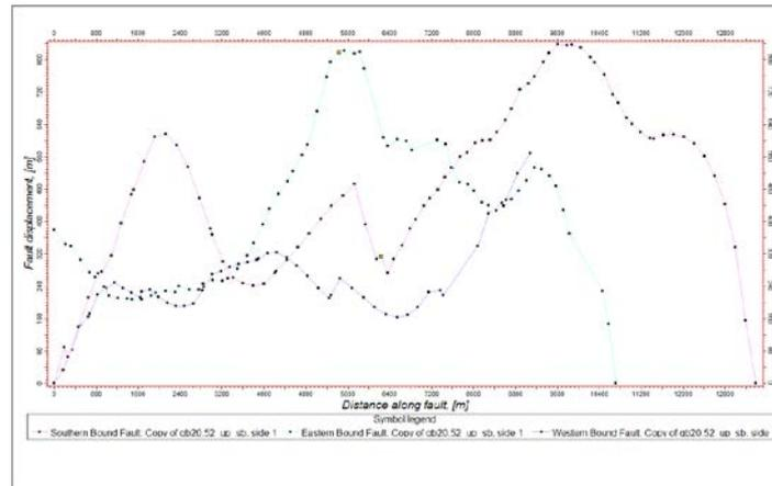
Fig.4: Fault displacement cross plot for Buselli main faults
