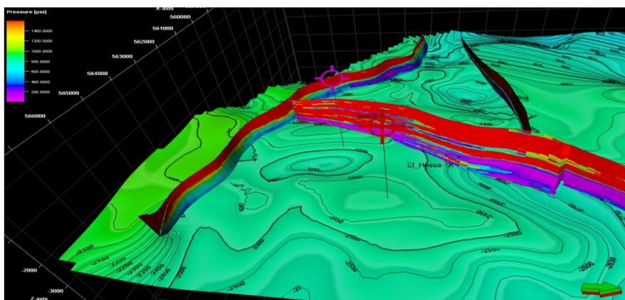
Fig.9: Threshold pressure distribution along the main bound faults.
