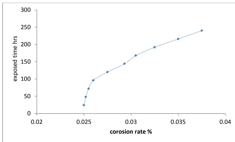
Fig.2. Rate of Corrosion with respect to Time
