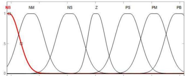
Fig.4.3 Input 1 Speed error membership functions
