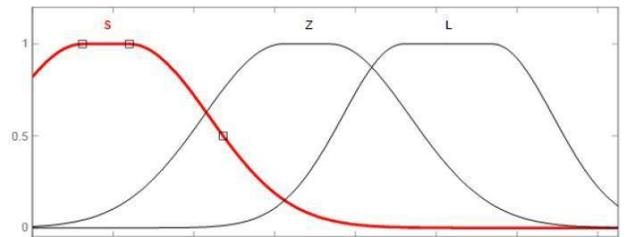
Fig.4.4 Input2 is current error membership functions
