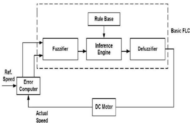
Fig.4.1 shows the basic structure of fuzzy logic controller.
