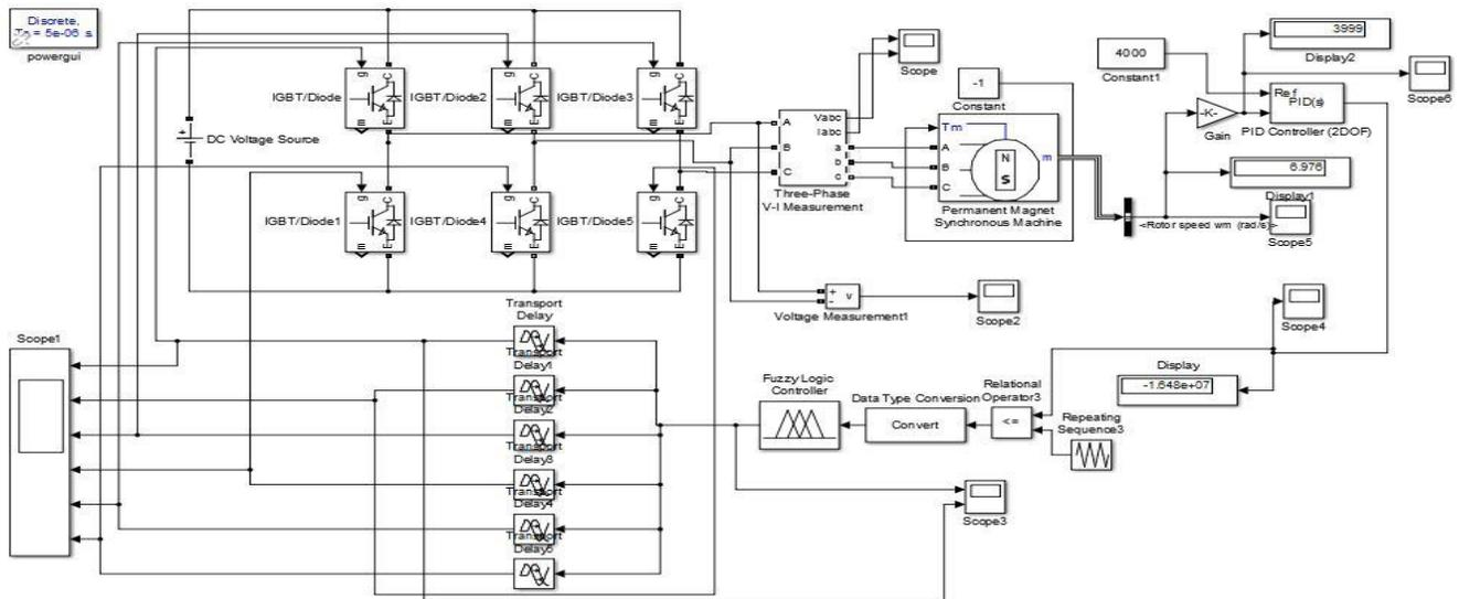
Fig.6.2 SIMULATION OF SPEED CONTROL OF PMSM USING FUZZY AND PID
