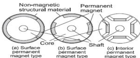
Permanent magnet synchronous motor structure
