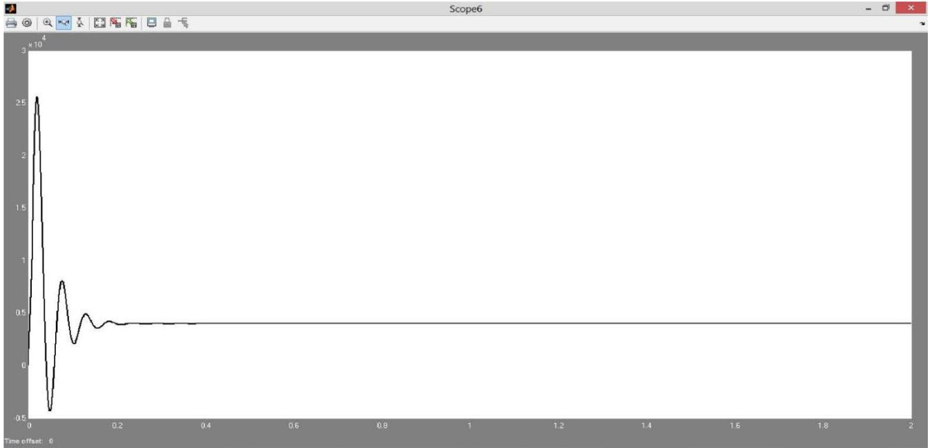
Fig.6.3 PMSM drive speed control with PID (Speed response curve)
