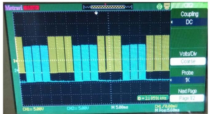
Fig 5.4 PWM pulses waveform
