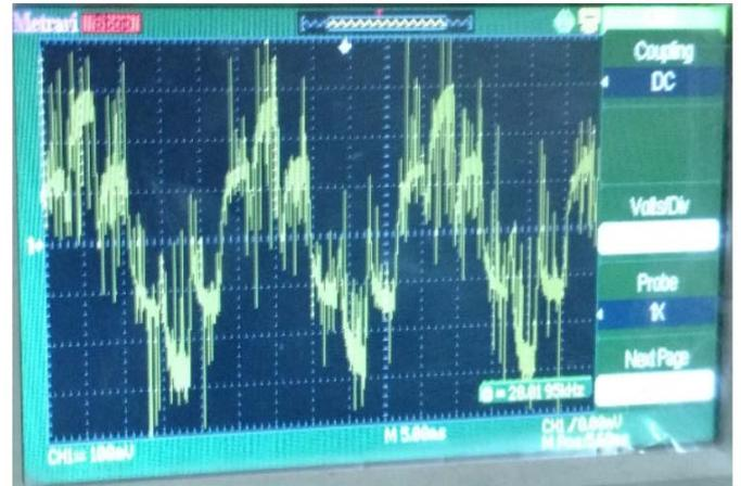
Fig 5.3 Stator current waveform
