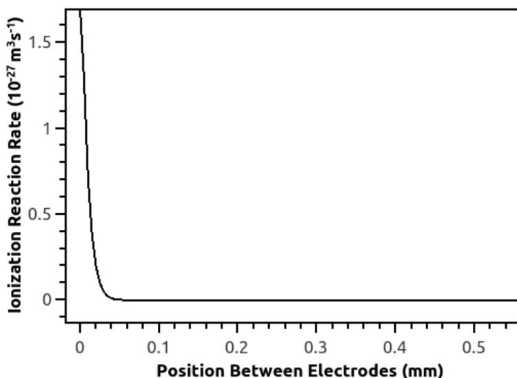
Figure 3: Average ionization reaction rate(S) between the electrodes in Helium DBD at Near Atmospheric Pressure for positive half cycle of 3535V AC supply.
