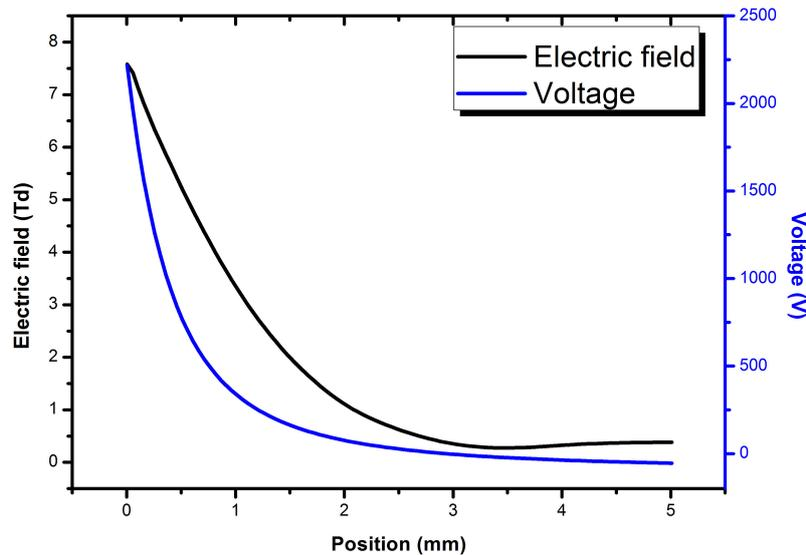
Figure 2: Average electrostatic potential between the electrodes in Helium DBD at Near Atmospheric Pressure for positive half cycle of 3535V AC supply.
