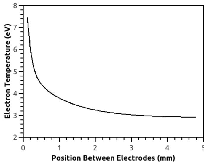
Figure 4: Average electron temperature ( $T_e$ ) between the electrodes in Helium DBD at Near Atmospheric Pressure for positive half cycle of 3535V AC supply.
