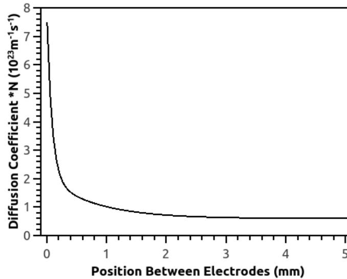
Figure 5: Average electron diffusion coefficient( $D_e$ ) between the electrodes in Helium DBD at Near Atmospheric Pressure for positive half cycle of 3535V AC supply.
