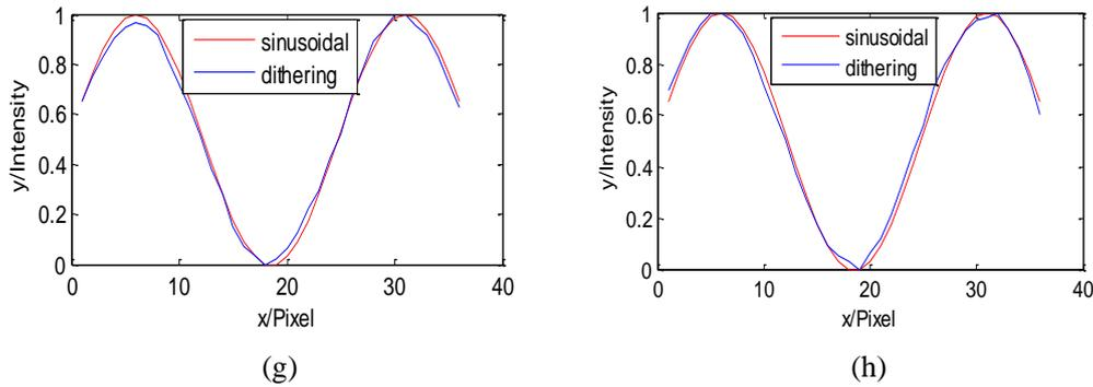
Fig.2 Sinusoidal comparison of dithered fringe patterns. (a)Bayer dithering; (b)Floyd-Steinberg dithering; (c)Sierra dithering; (d)Burkers dithering; (e)~(h)Sinusoidality of dithered fringe patterns after defocusing(with filter size 5 and fringe period 25)
