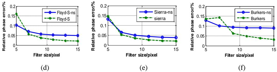
Fig.5 Effects of different filters for different scanning paths on T=25 and T=100. (a)~(c)T=25; (d)~(f)T=100
