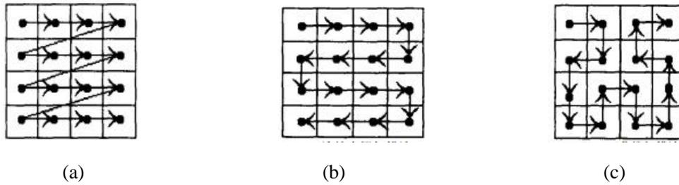
Fig.1 diagram of different scanning paths. (a)horizontal scanning; (b)spiral scanning; (c)Hilbert scanning
