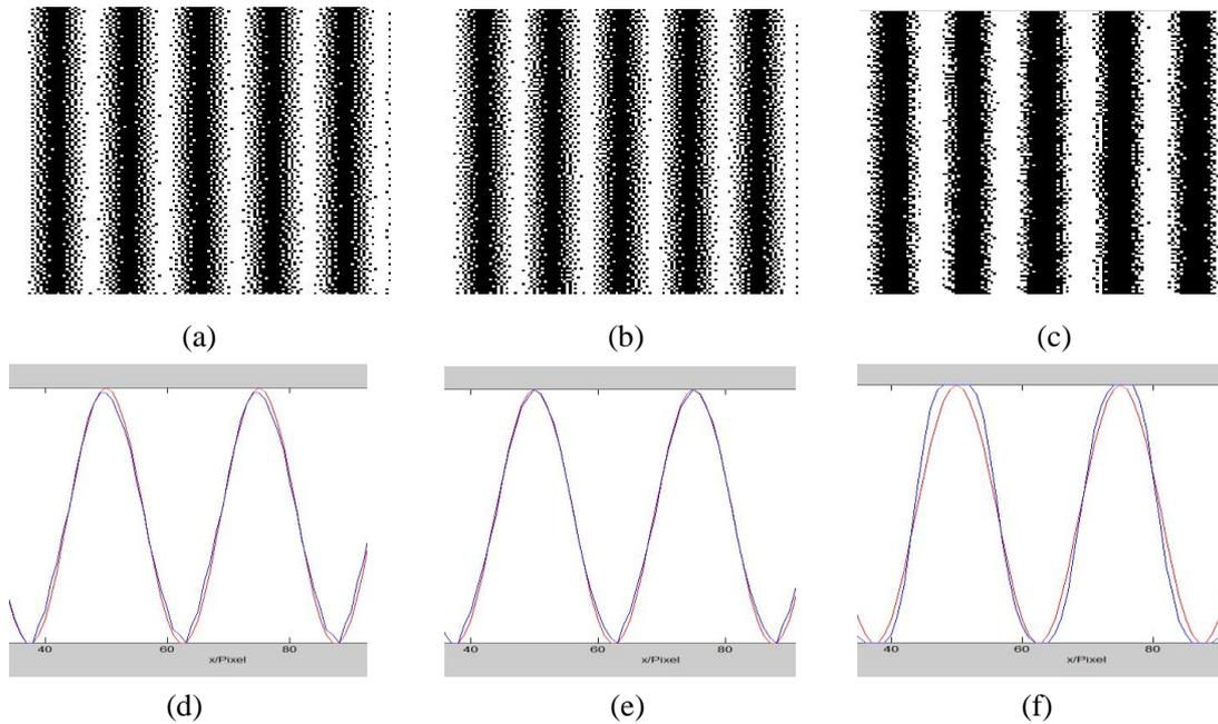
Fig.4 Sinusoidal comparison of dithered fringe patterns.(a)Floyd-Steinberg dithering on horizontal sweep; (b)Floyd-Steinberg dithering on helical sweep; (c)Floyd-Steinberg dithering on Hilbert sweep; (d)~(f)Sinusoidality of dithered fringe patterns after defocusing(with filter size 5 and fringe period 25)
