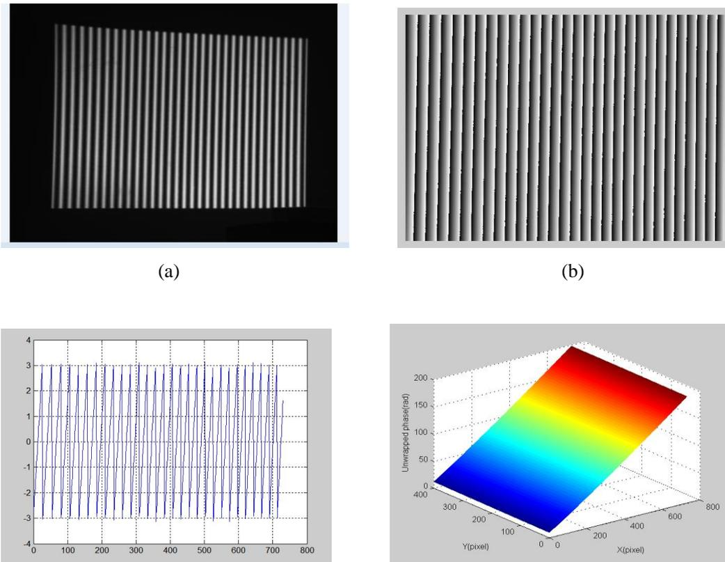
(c)the cross-section of the main value of the phase (d)unwrapping phase
