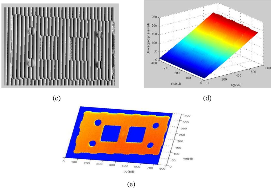
Fig.8 Measurement of an object with Sierra dithered fringe pattern on helical sweep. (a) object to be measured; (b) one of four-step phase-shifting fringe pattern; (c) wrapped phase; (d) unwrapped phase; (e) final phase of the object
