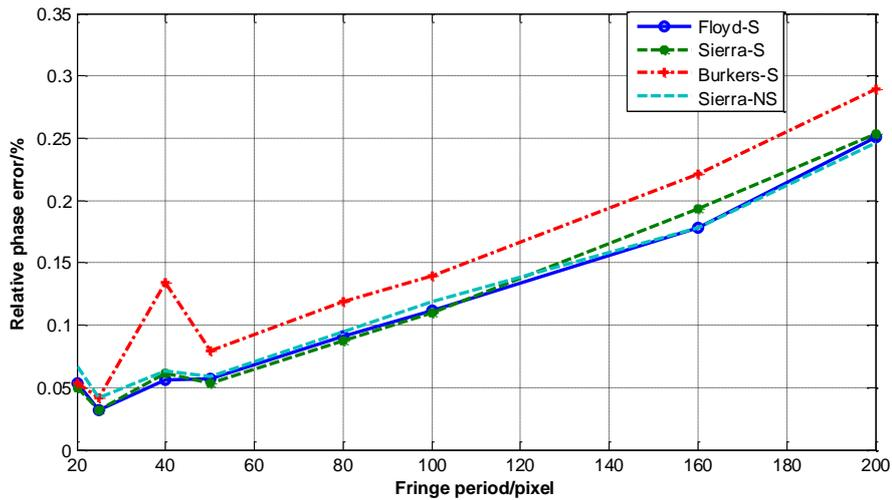
Fig.7 Relative phase error of different filters on helical sweep
