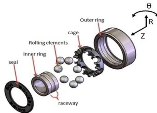
Fig.1. components of rolling element bearing
