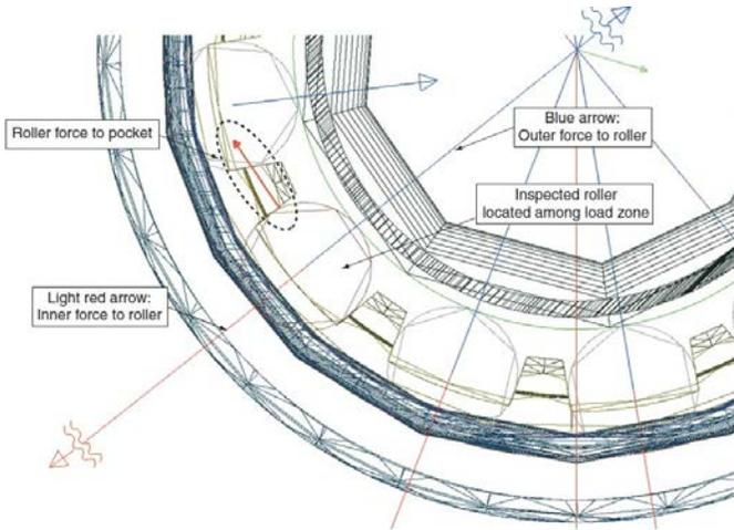
Fig.3. loads on outer race
