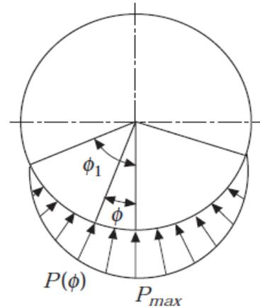
Fig.2. Load on rolling element bearing
