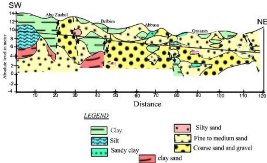
Fig. (5) Hydrogeological cross section along the right bank of Ismailia canal
