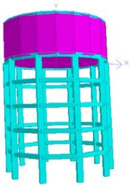
Staging without inclined bracing
