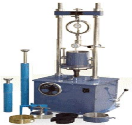
Fig.2 Equipment for swelling pressure test
