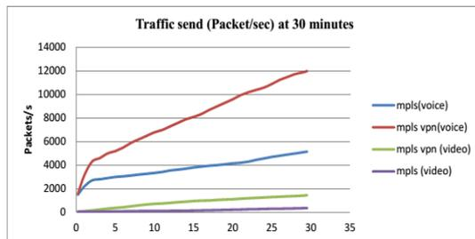
Fig (10): Traffic Sent (Packet/s) at 30 minutes
