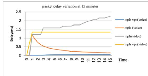
Fig (5): Packet delay Variation at 15 minutes
