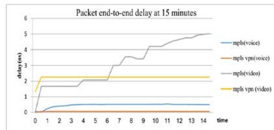
Fig (7): Packet End-to-End Delay at 15 minutes
