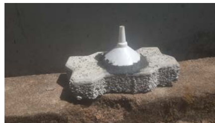
Fig 3: (a) lab setup for permeability test (b) pervious interlock casted for test
