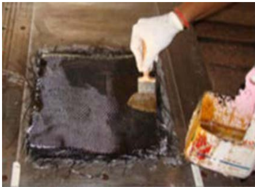
Fig. 3.4 Hand layup process
