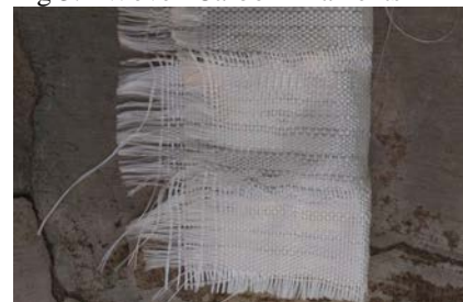
Fig3.2 Woven Glass filaments
