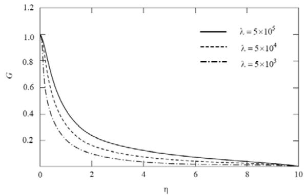
**Figure -3: Temperature profile for Pr=0.7**
