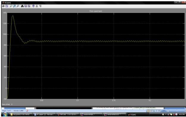
Fig. 6 motor speed waveform with boost converter
