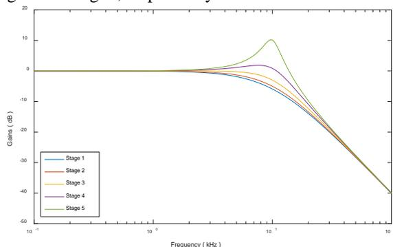
Fig. 3 Gain curves of each filter stage obtained by DE
