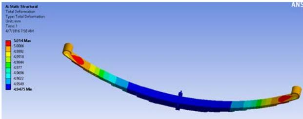
Fig.9 Total deformation
