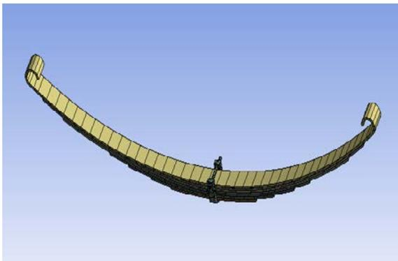
Fig.4 Meshing of spring
