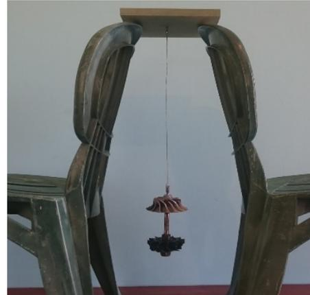
Fig. 5: Experimental setup to measure the inertia of the turbocharger rotor
